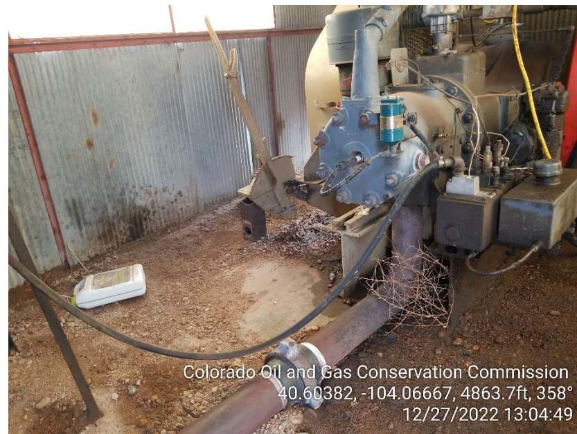
Photo 12 – Stained Soil at Gas Engine
