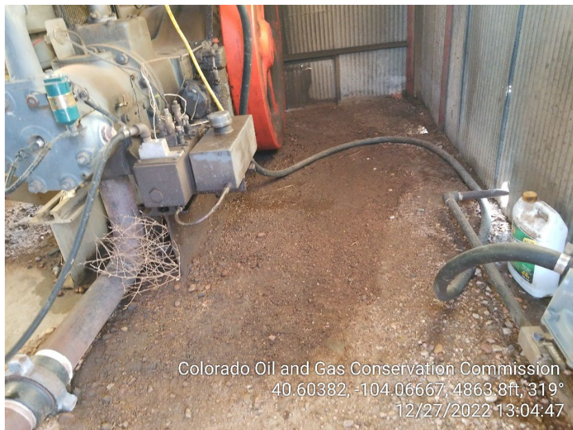
Photo 11 – Stained Soil at Gas Engine
