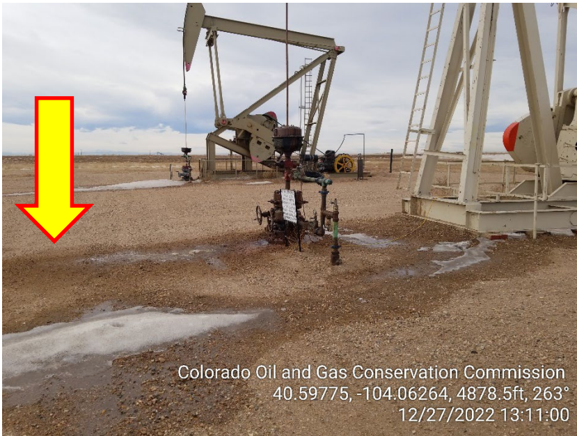
Photo 5 – Stained Soil at 2-6 Wellhead
