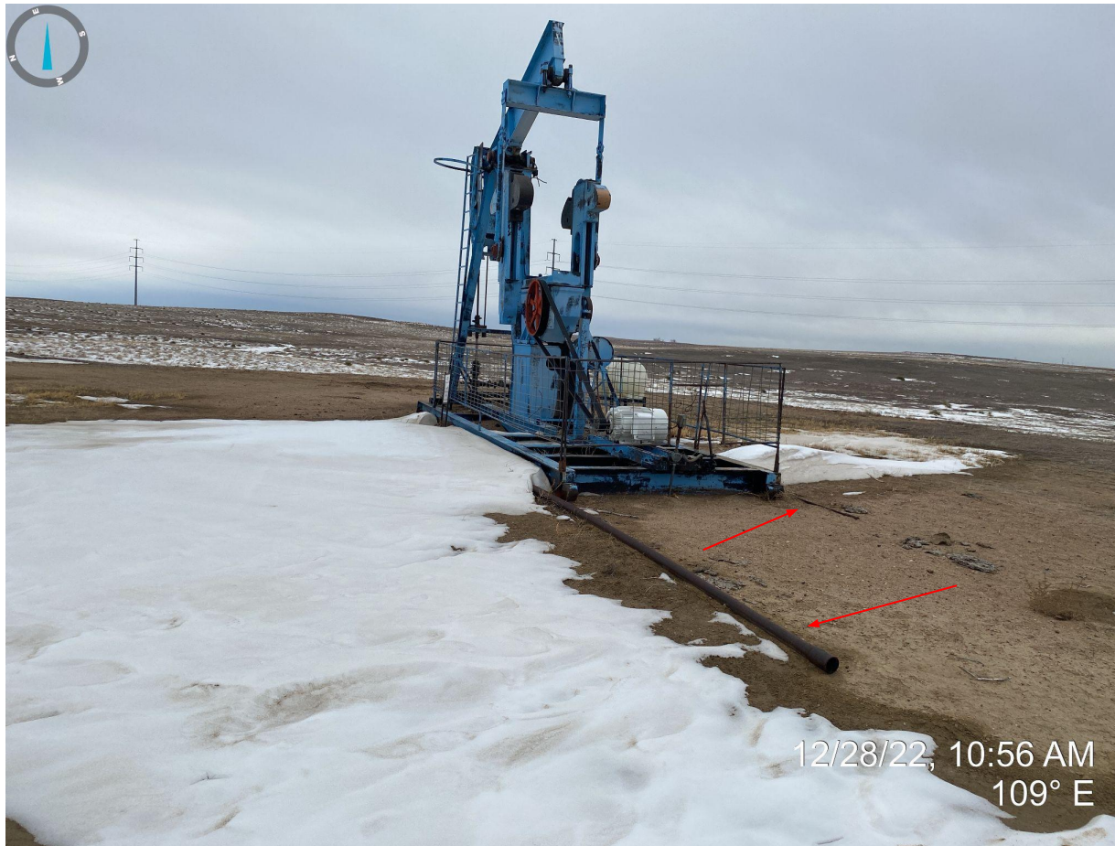
Photo 1. Facing east from western portion of location. Photo shows unused equipment (e.g. pipe and sucker rod) on location. This is considered unused equipment and needs to be removed.
