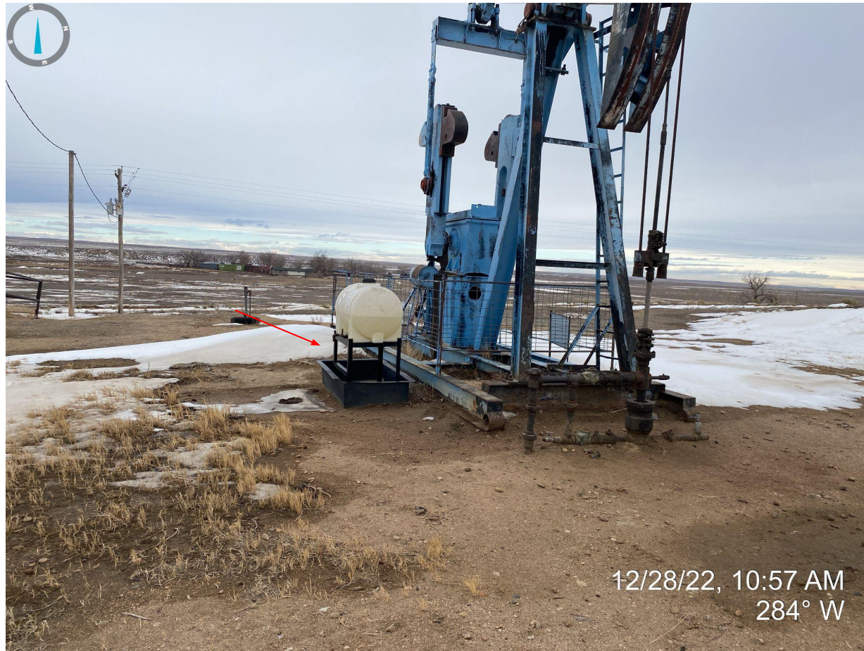
Photo 3. Facing west from the eastern portion of the well location. Red arrow illustrates no visible netting/wildlife protection around open tank.
