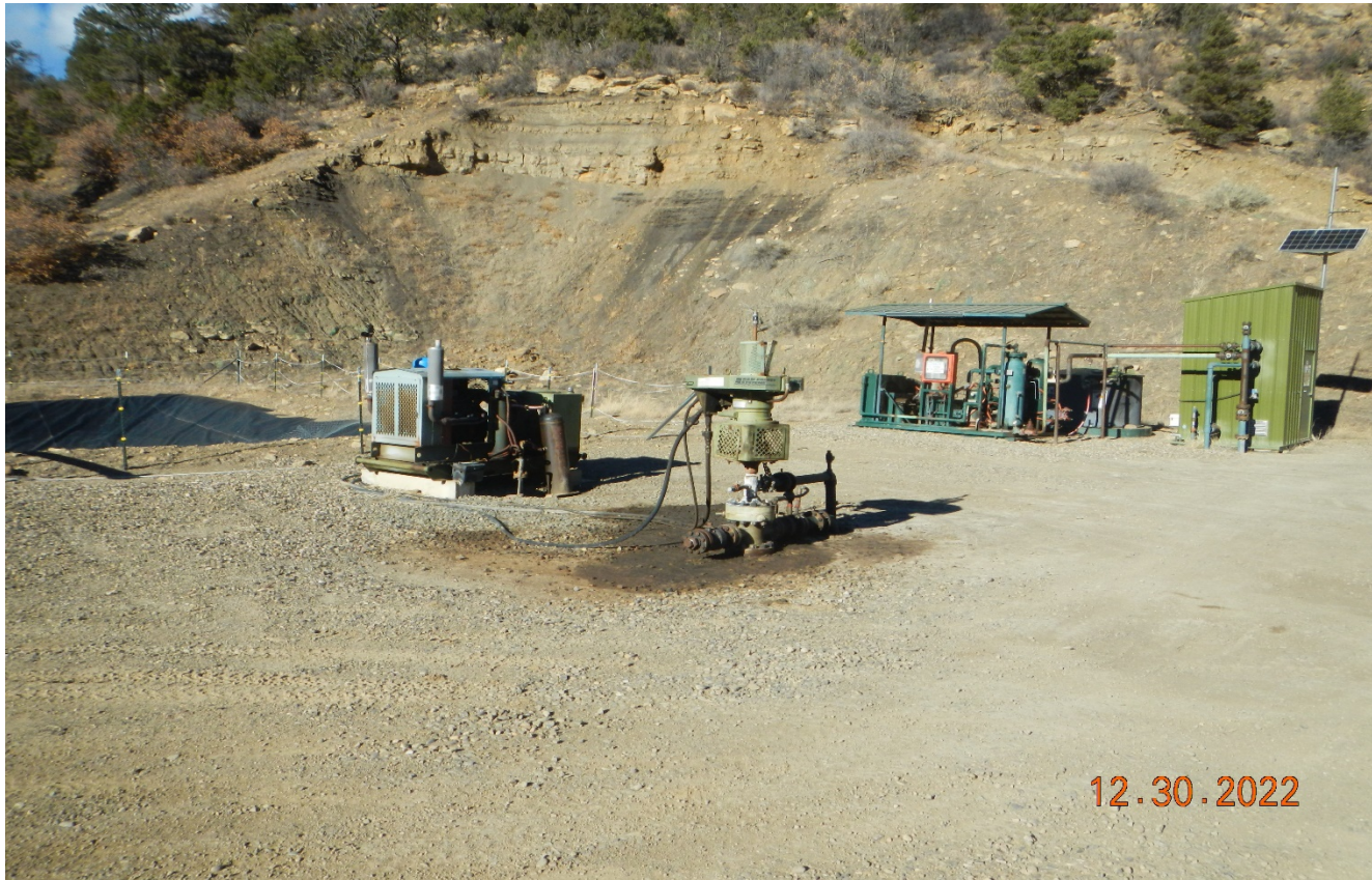
Photo 1. Facing toward the wellsite. There is oil stained soil around the wellhead.
