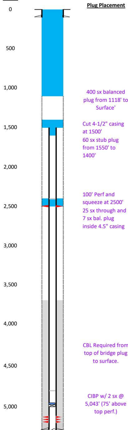
CBL Required from top of bridge plug to surface.
