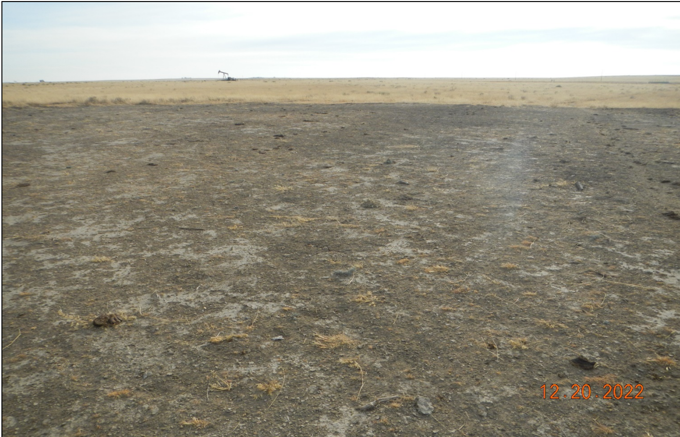
Photo 2. Facing south toward the location. The location has been recontoured and decompacted. Soils have not been seeded and stabilized.
