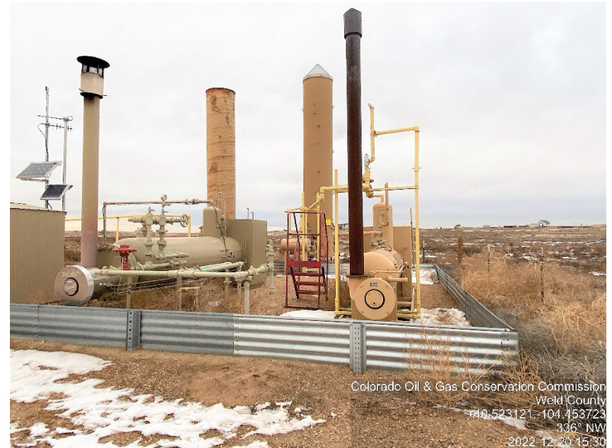
Photo #4 Turman 32-42 Battery site Active Separators, ECDs
