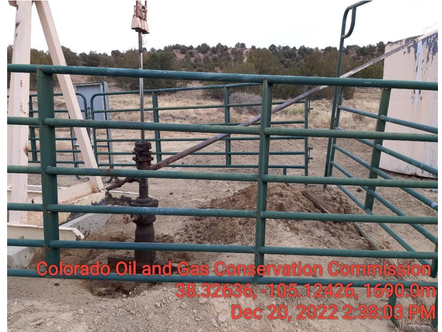
Photo 2 Well head stained soil and no braden head not plumbed to surface
