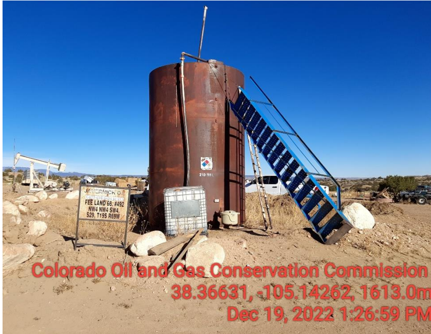
Photo 3 Stairs in disrepair considered unused equipment. Trash : rocks wood dead weeds. Plastic tote unused equipment
