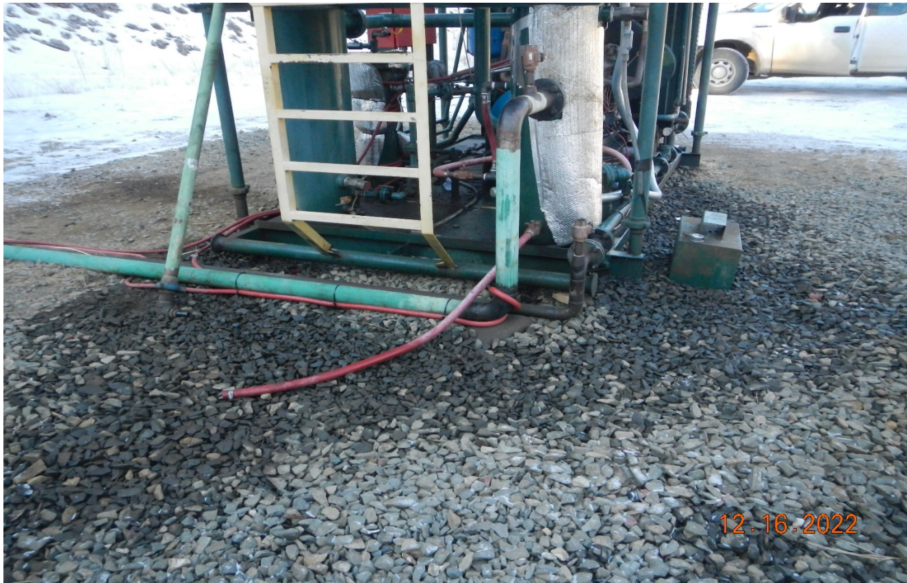
Photo 3. The engine compressor appears to be leaking oil which has spilled over on the surface.
