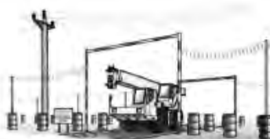
EXAMPLE OF GOAL POST INSTALLED PERPENDICULAR
