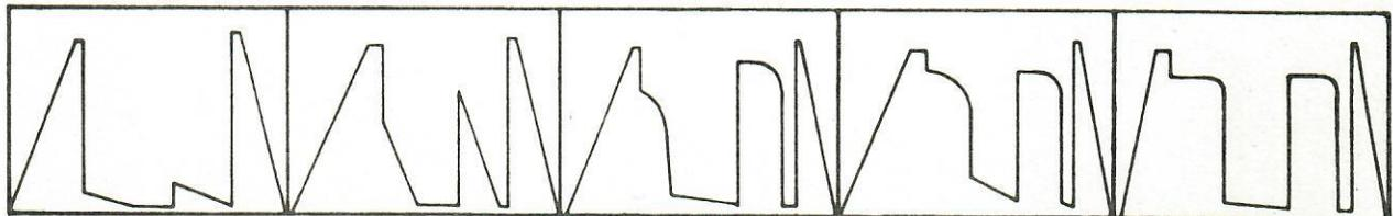
Very low permeability. Usually only mud recovered from interval tested. Virtually no permeability.
