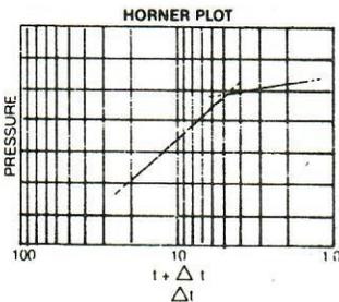
**Horner Plot Slope Breaks Downward**
