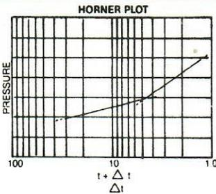
**Horner Plot Slope Breaks Upward**
