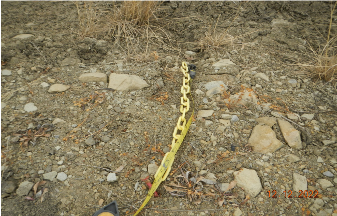
Photo 6. The freeboard marker is not is not 2ft. In length and does not show the vertical depth where it is installed. (Lays horizontal on the ground)
