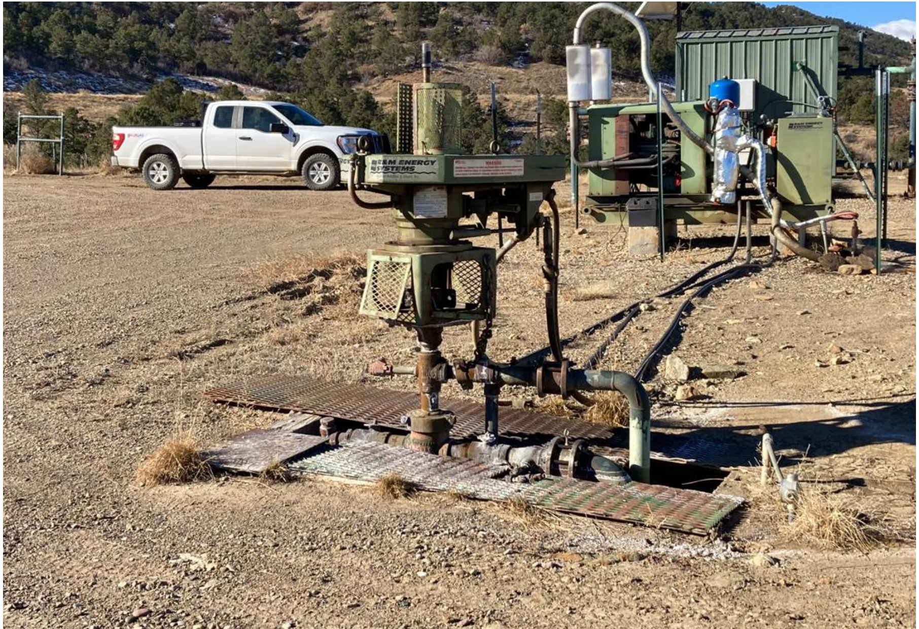
PHOTO 1: THE WELLHEAD PACKINGS WERE REPLACED AND THE STUFF BOX WAS SECURELY FASTENED TO STOP THE WATER LEAK. THE SELF INSPECTION PROCESS HAS BEEN REVIEWED.
