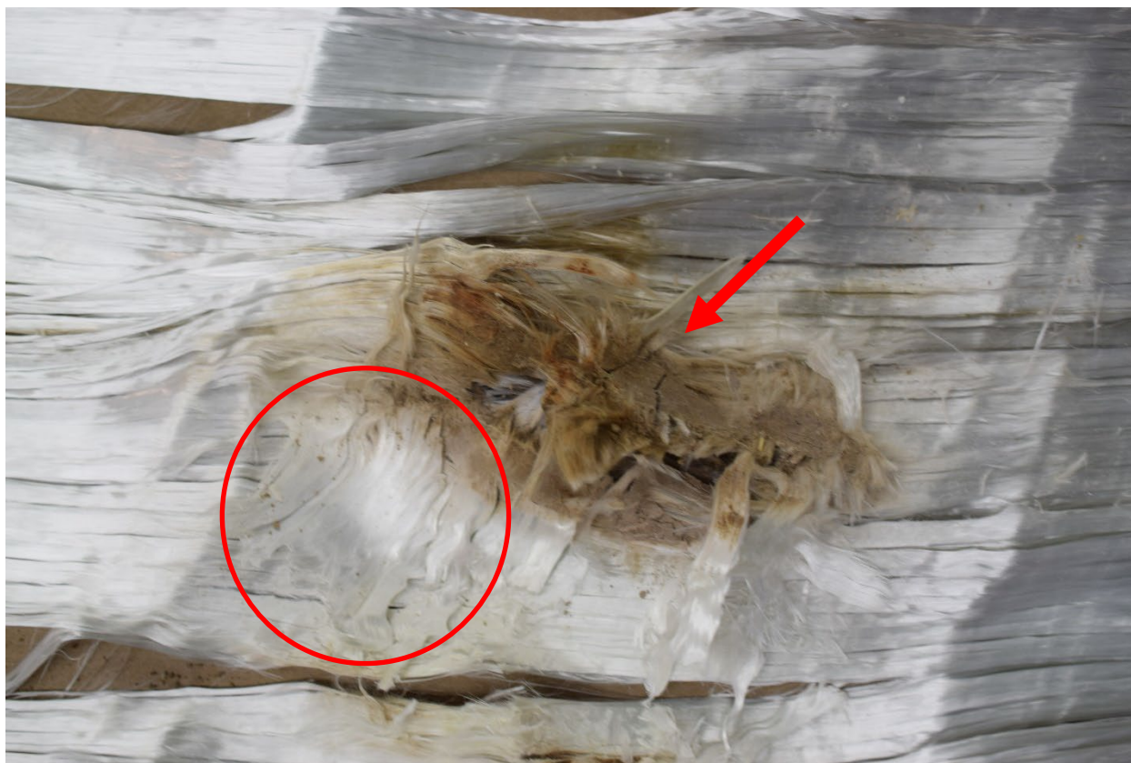
Figure 9. Inner view of the outer fiberglass reinforcement layer following removal from the liner. Note main rupture location at red arrow and broken inner fiberglass reinforcement layer pieces at red circle. Also note uniformity of fiberglass reinforcement just outside of the rupture location.
