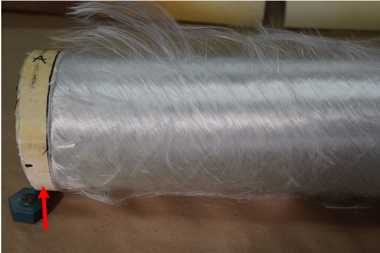
Figure 8. Fiberglass reinforcement at one end of the rupture section following removal of the outer jacket. Note uniformity of the reinforcement layer just outside of the rupture location.
