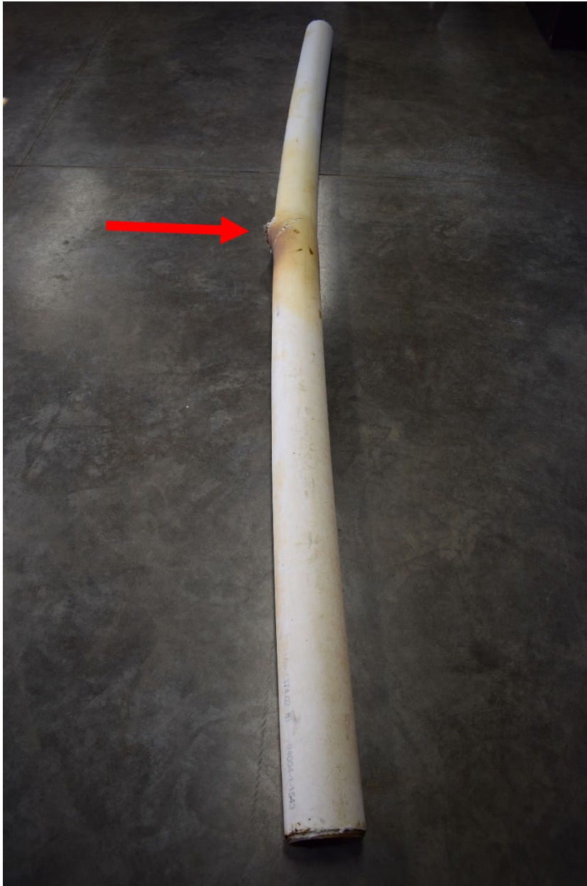
Figure 1. Ruptured sample as-received. Note failure location at approximate mid-length of the sample indicated by red arrow.
