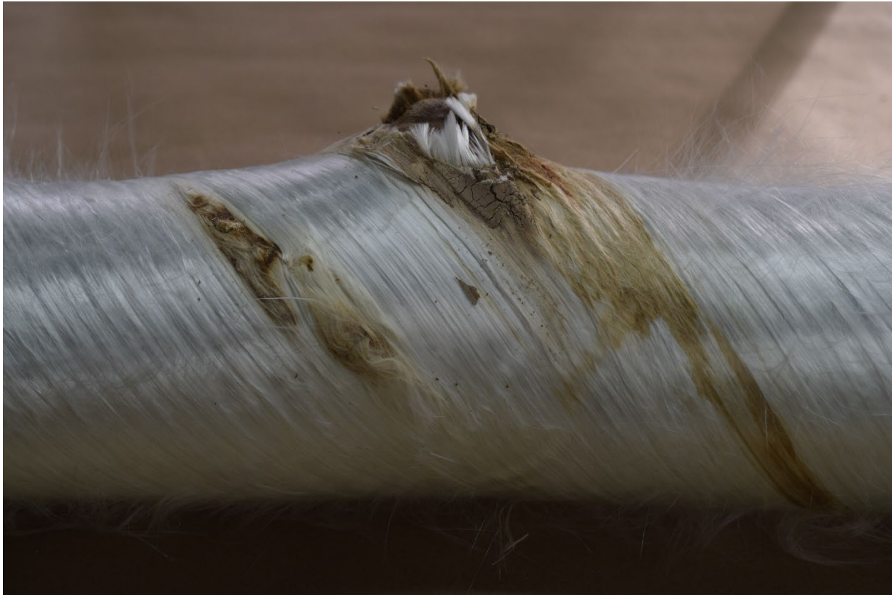
Figure 7. Close-up image of the rupture location with the outer jacket removed. Note separation of the outer fiberglass reinforcement surrounding the leakage locations.
