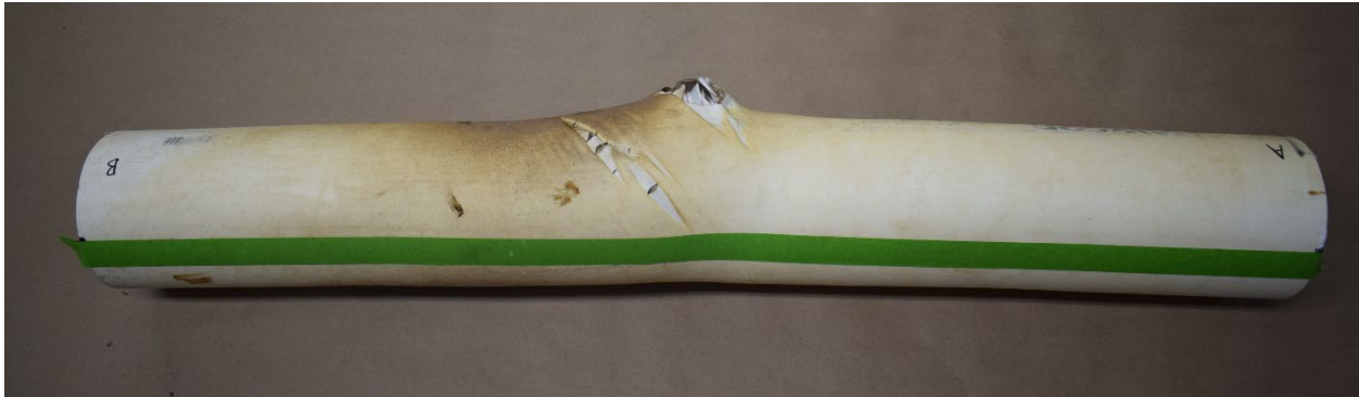
Figure 5. The 3-foot-long section following marking with masking tape. Note that another line is marked approximately 180° opposite the one shown.
