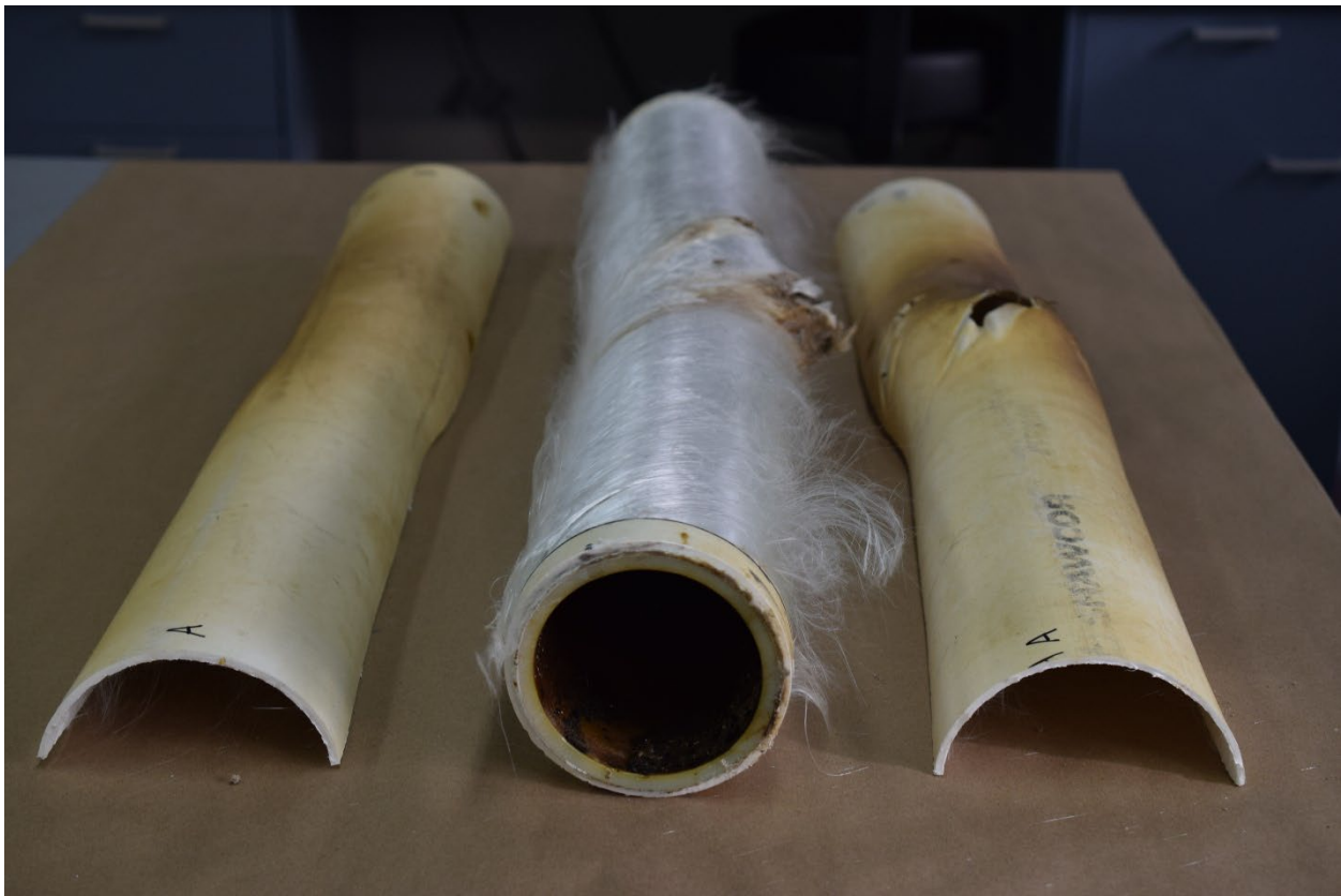
Figure 6. The rupture section following removal of the outer jacket.
