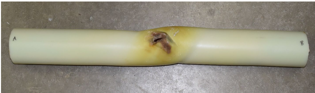
Figure 11. HDPE liner following removal of the fiberglass reinforcement layers. Note rupture and discoloration at the center of the liner section.
