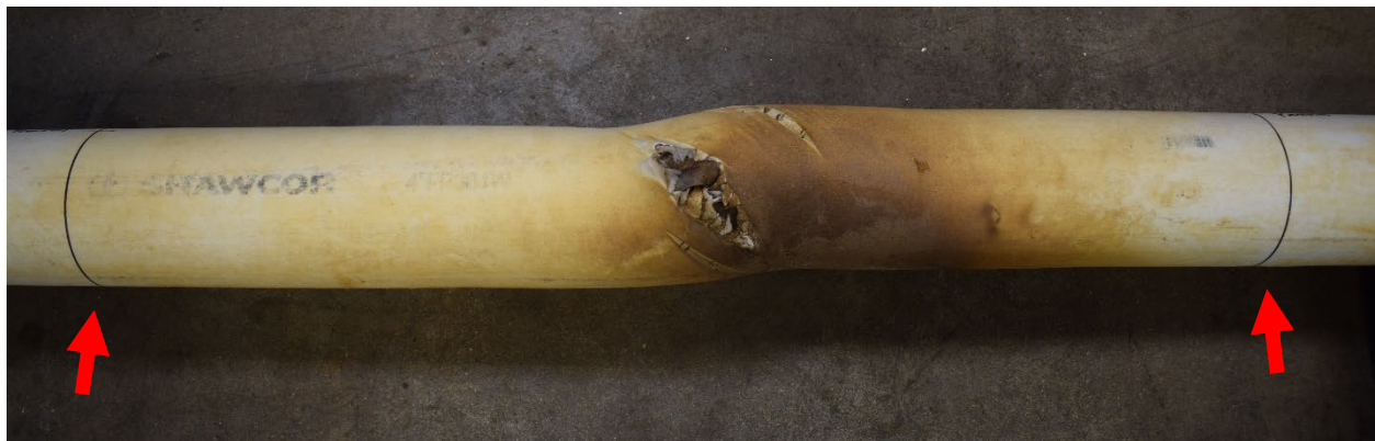
Figure 4. The 3-foot-long section of the rupture sample marked prior to cutting.
