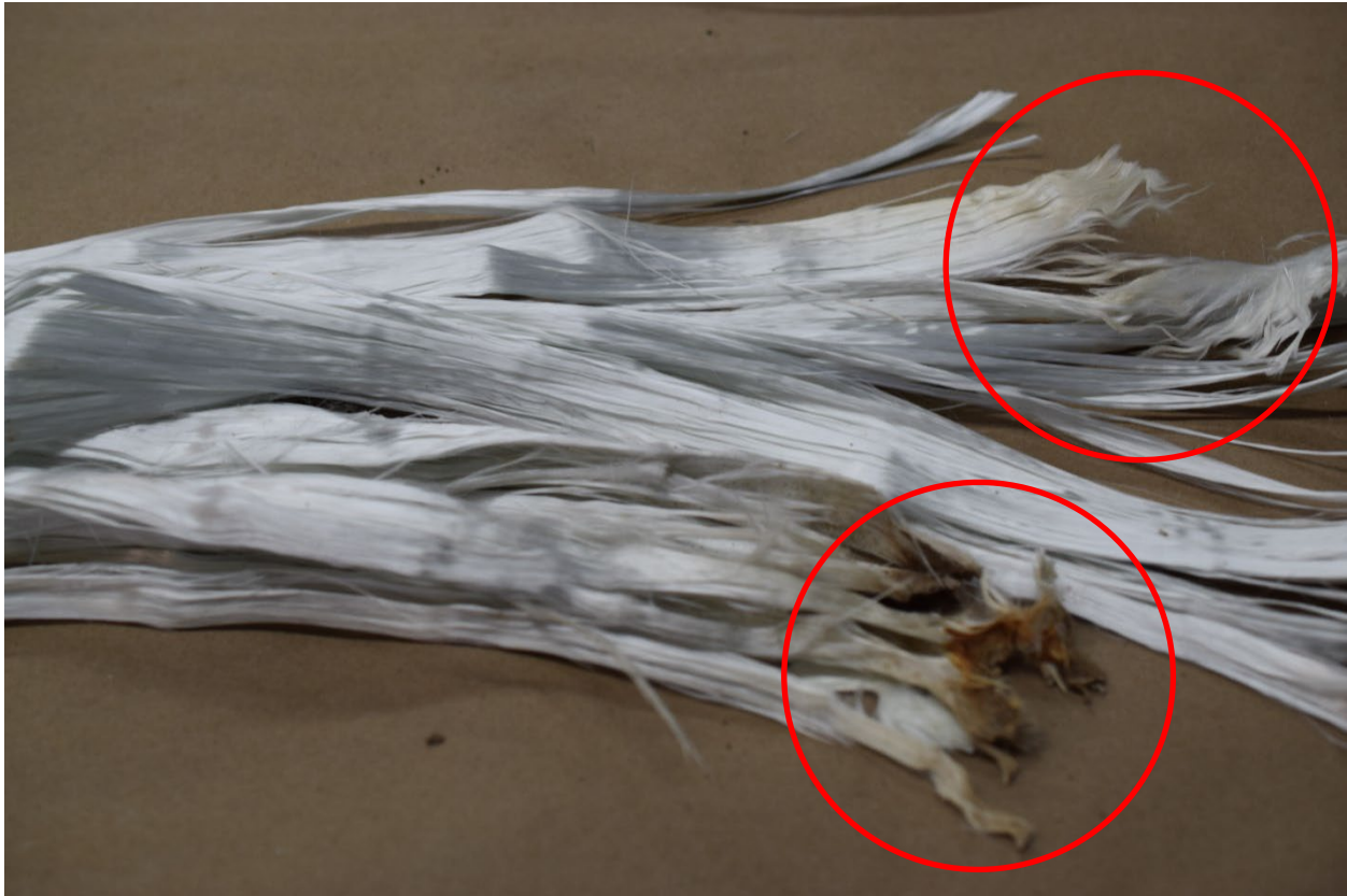
Figure 10. Inner view of the inner fiberglass reinforcement layer following removal from the liner. Note random, i.e., not straight or aligned, breaks of the fiberglass reinforcement layer at red arrows.
