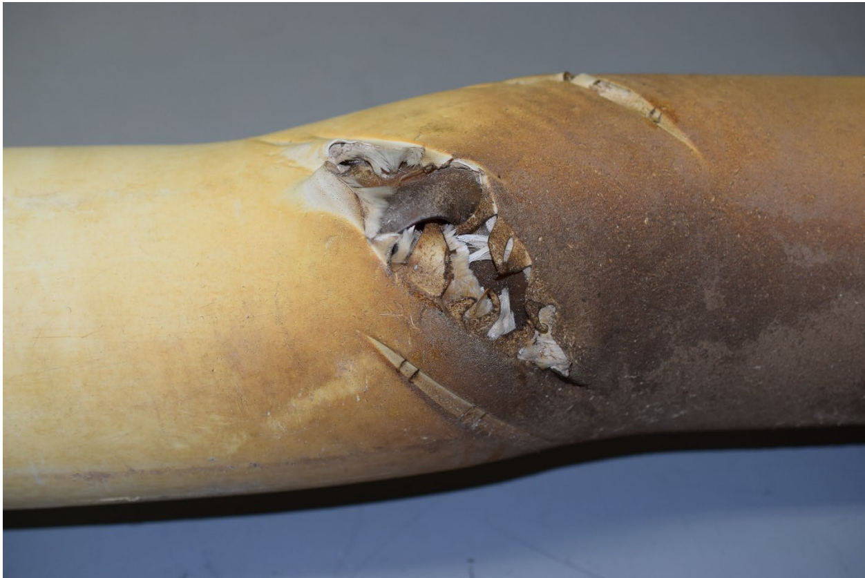
Figure 2. Close-up image of the failure location on the ruptured sample shown in Figure 1. Note pipe axis deviation centered on the failure locus.
