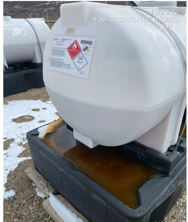
Photo 3. Photo taken from the well area shows one of two leaking corrosion inhibitor tanks.
