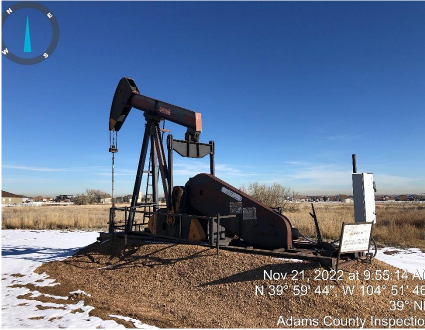
Photo#1 Pump Jack.
