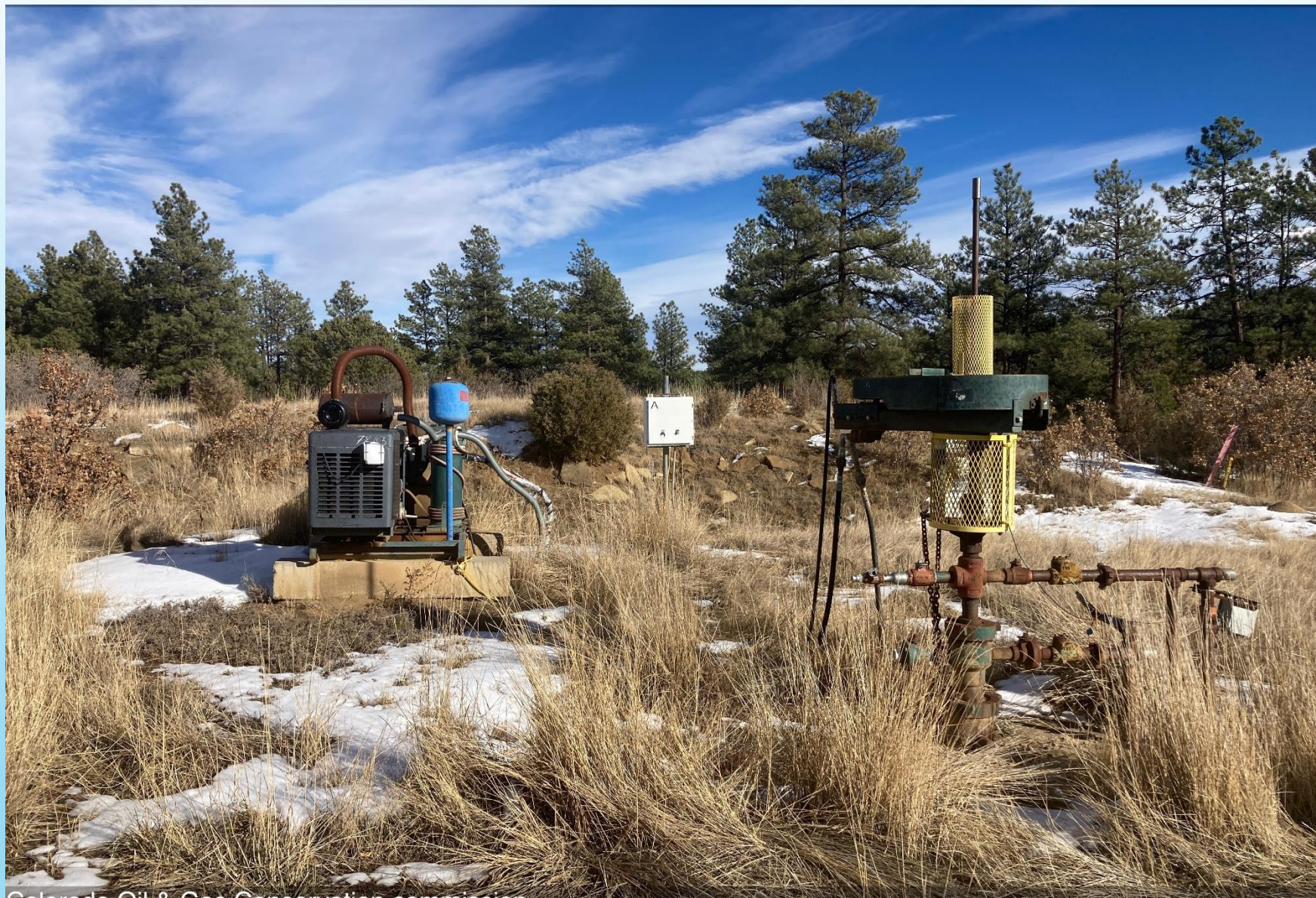
PHOTO 3: WELLHEAD AND EQUIPMENT
