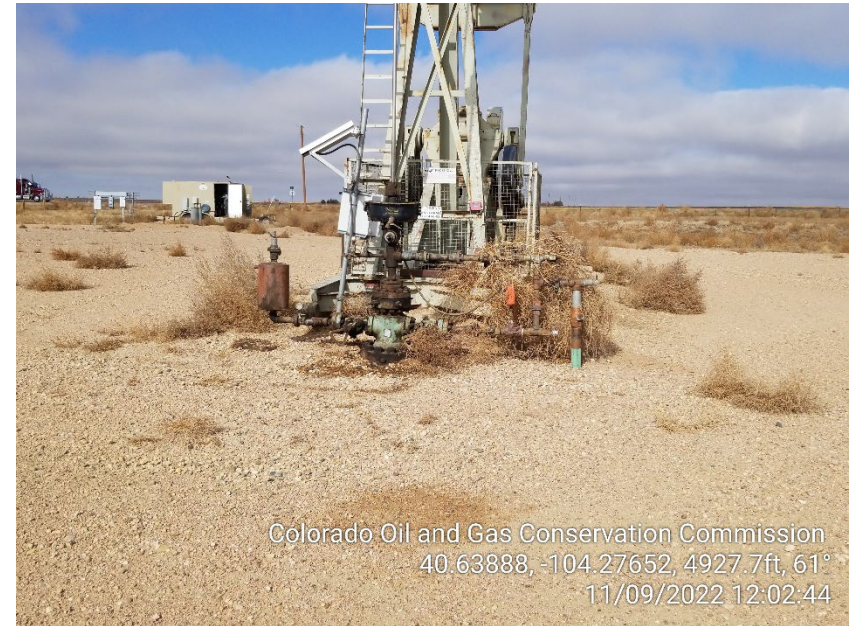
Photo 4 – Wellhead – Stained Soil
