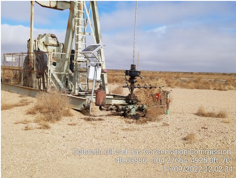
Photo 3 – Wellhead – Stained Soil
