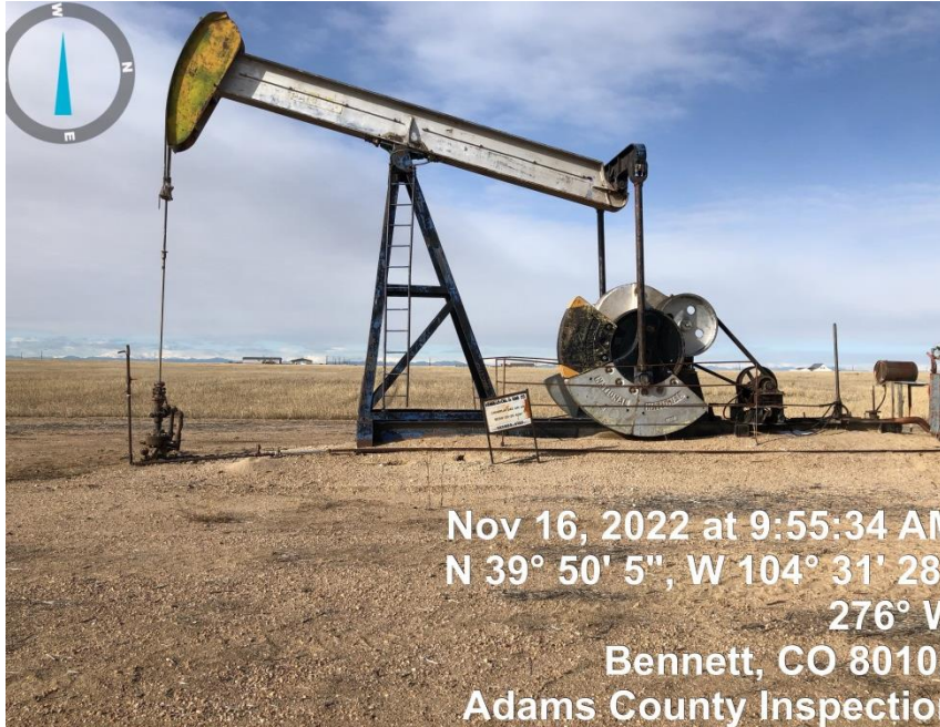
Photo#1 Pumpjack/Wellhead
