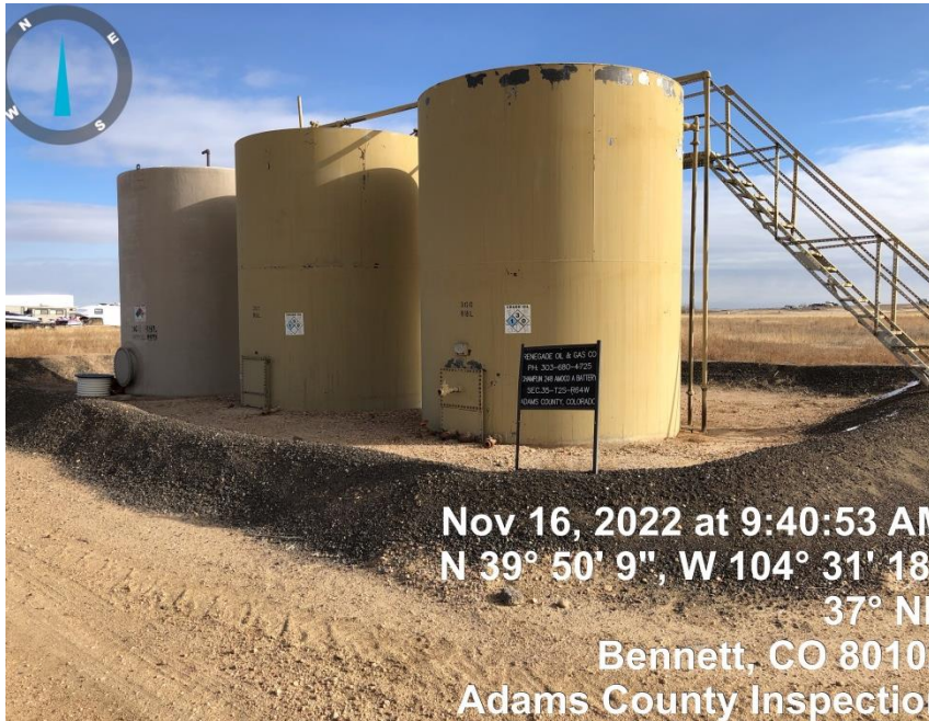
Photo#1 Production Tanks & Produced Water Tank
