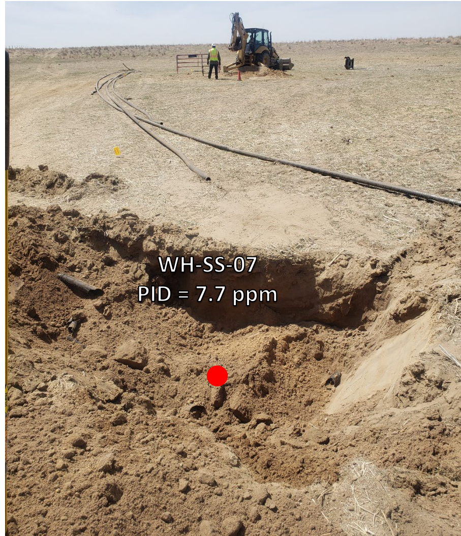
Looking west at flowline change in direction No petroleum hydrocarbon staining or odor observed
