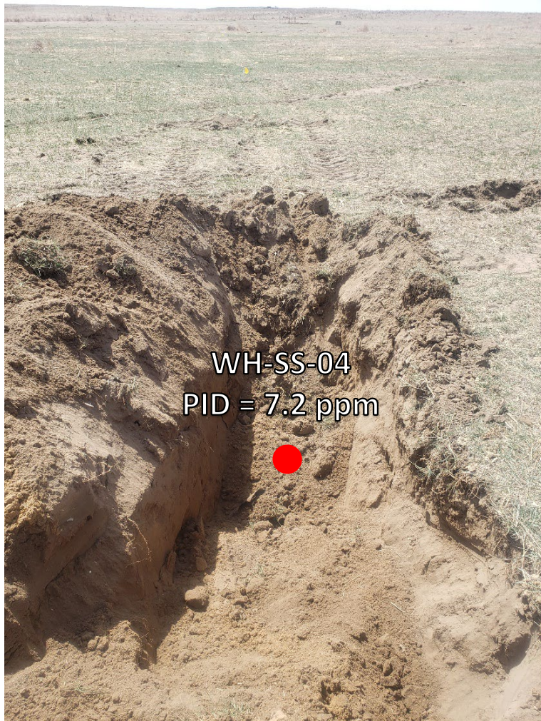
Looking southwest at cut point No petroleum hydrocarbon staining or odor observed
