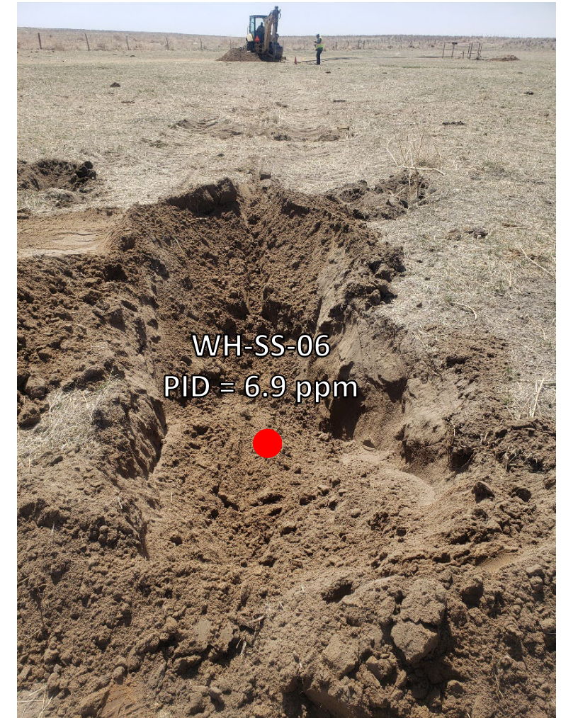
Looking southwest at cut point No petroleum hydrocarbon staining or odor observed
