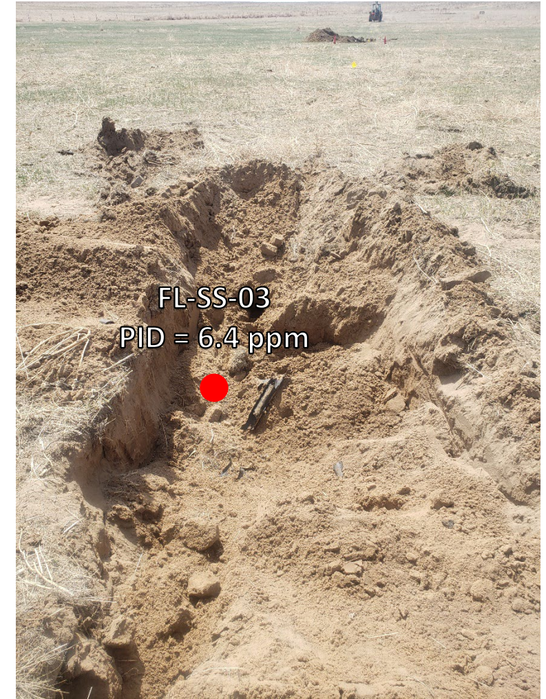
Looking south at cut point No petroleum hydrocarbon staining or odor observed
