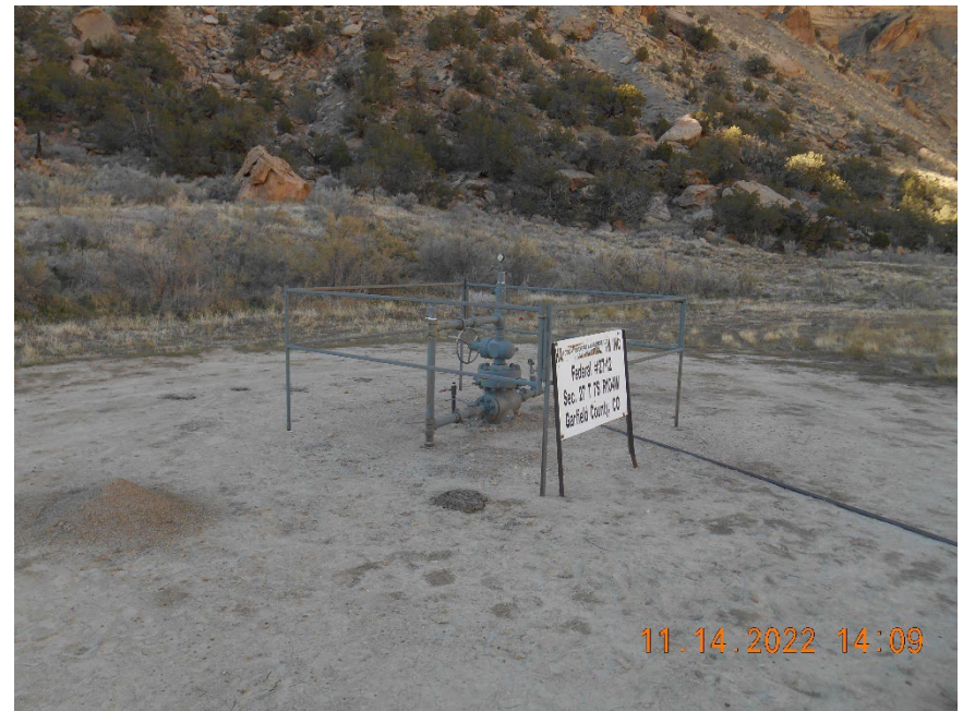
Wellhead with improper sign
