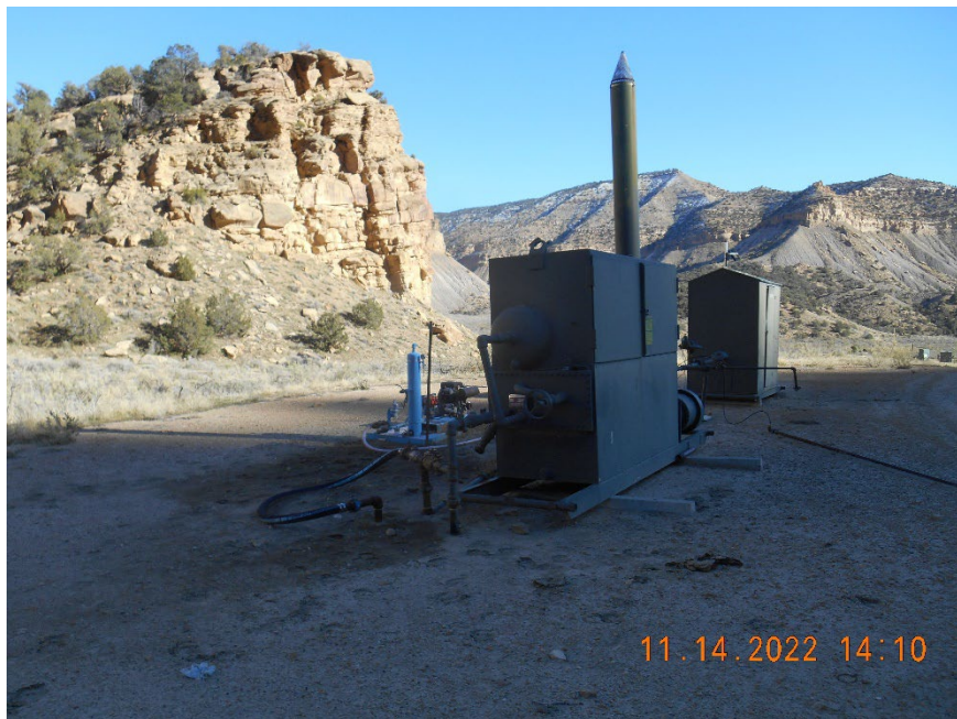
Meter housing, Separator & compressor
