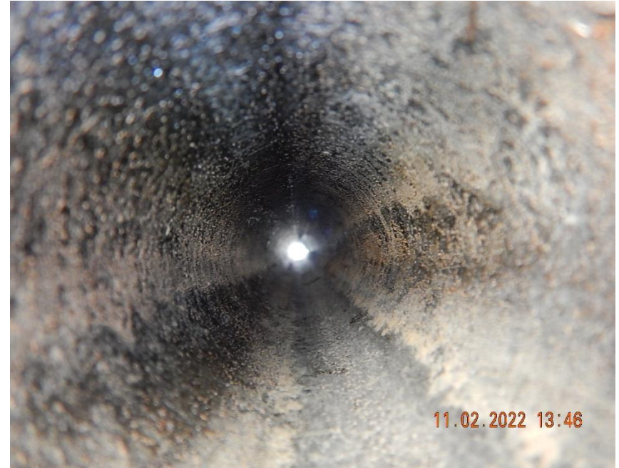
Internal photo of failed section of MSSU 19-5 flowline pipe.
