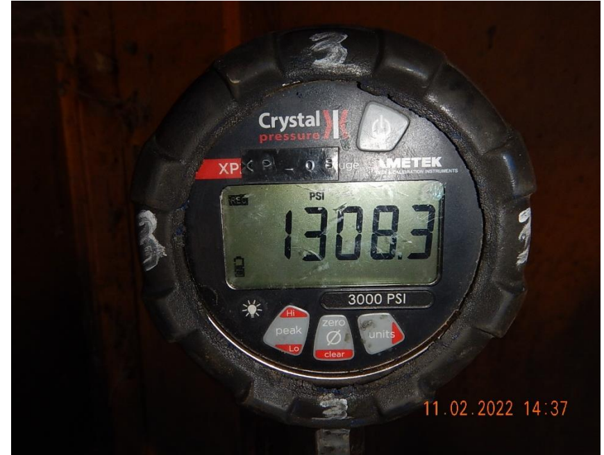
Flowline pressure test witnessed; crystal gauge reading near end of pressure test (verification of repairs completed).
