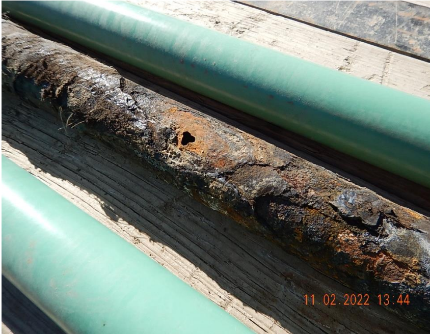
Corrosion hole identified on flowline pipe; MSSU 19-5 PW Injection flowline (off location). Coating damage observed in area of failure.
