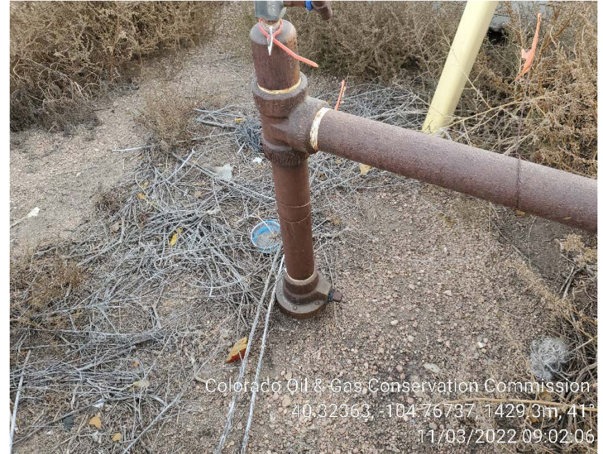
Wellhead Balon valve and riser
