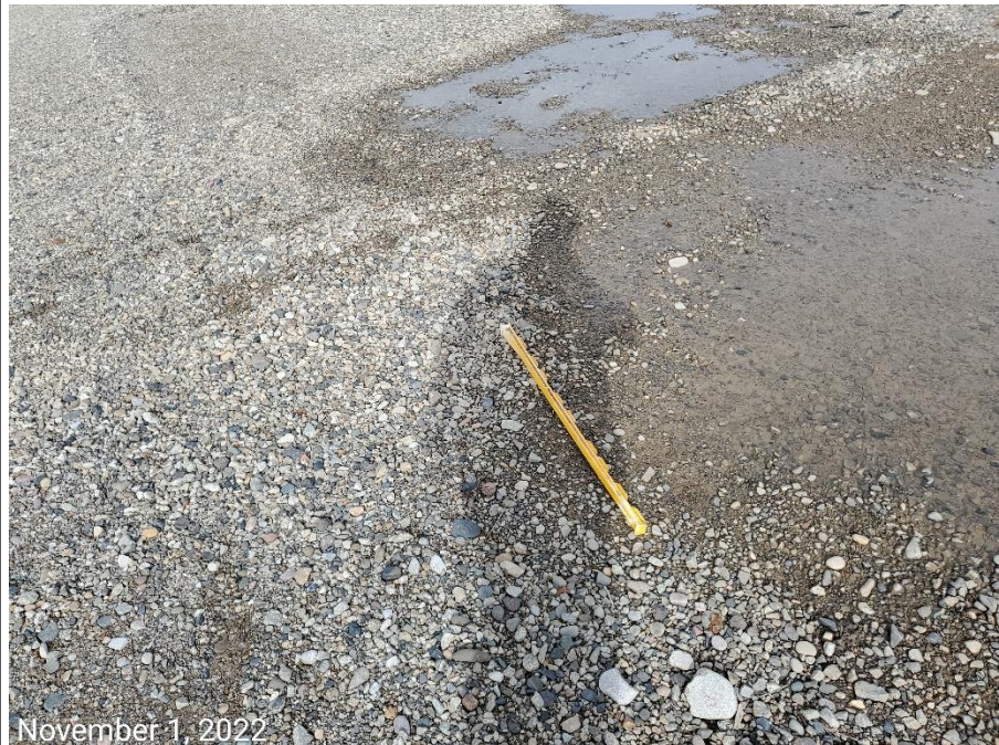
Photo 11: Photos examples showing markers at anchors not in proper functioning condition. Maintenance required. Unable to find anchor associated with marker observed in left photo.
