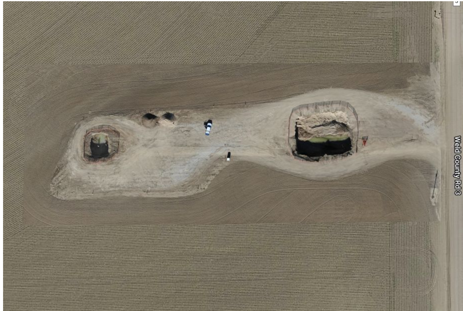
Photo 1. COGCC drone aerial imagery taken on 11/2/2022 illustrating the active remediation projects related to the Halverson 1 well. Photo illustrates an open remediation for the wellhead and tank battery.
