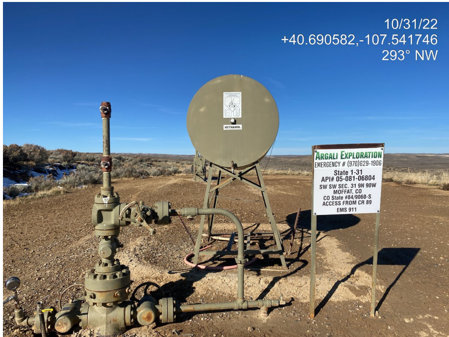
Photo 2. Photo shows production equipment. Secondary containment for the methanol tank is degraded and insufficient. Signs on Location have been updated with current Operator information.
