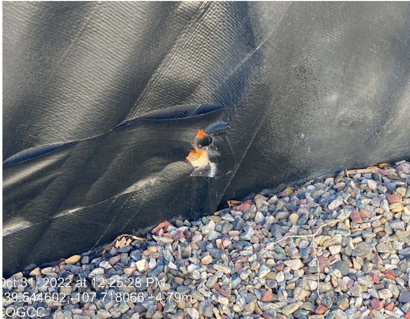
Holes in containment
