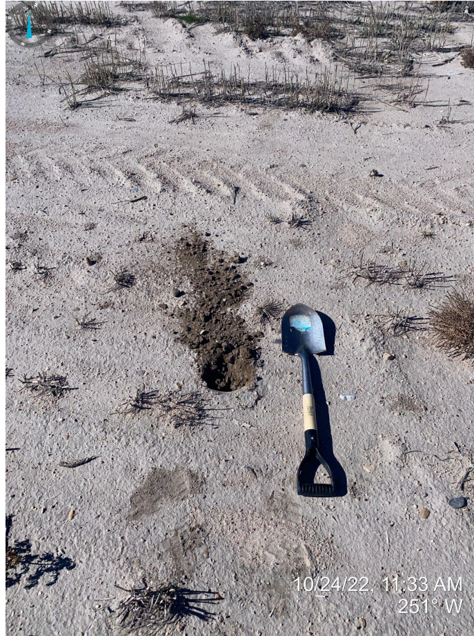
Photo 4. Close up photo taken from location. Photo illustrates the location has not been decompacted (hole dug approximately 3” before compaction was reached).
