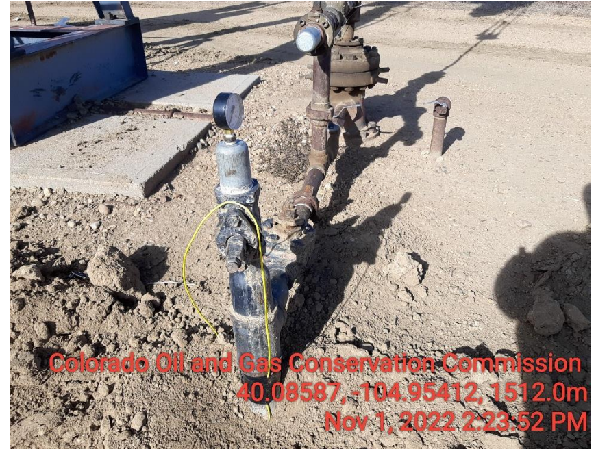
Photo 4 locating wire on flowlines
