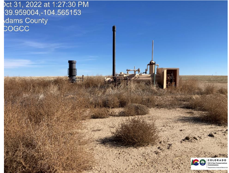
Pic 2 separator, ECD, weeds unmanaged.
