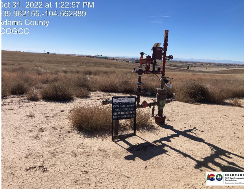
Pic 1 wellhead
