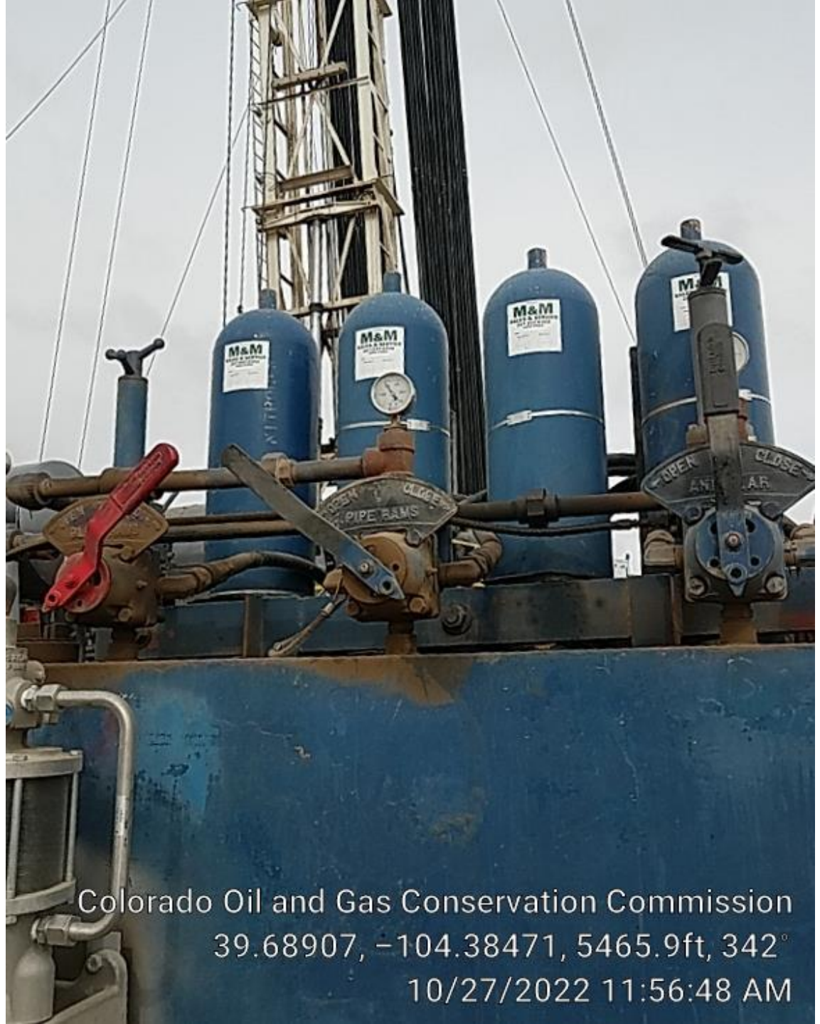
Accumulator/pipe rams at 2000 psi
