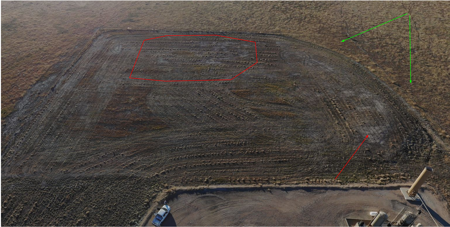
Photo 1. Drone aerial imagery illustrates the pit area. Bare patches were observed throughout (red arrow and polygon show examples of some of the bare patches) and weedy, annual vegetation was observed that is not reflective of reference areas. Desirable establishment was observed but introduced plant species were observed along the eastern interim and pit areas. Photo also illustrates the location has been recently mowed. Green arrow indicates where COGCC Staff located reference area vegetation.
