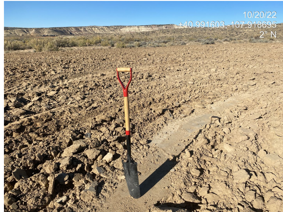
Photo 7. Photo shows shovel unable to penetrate a continuous unripped strip of soil.
