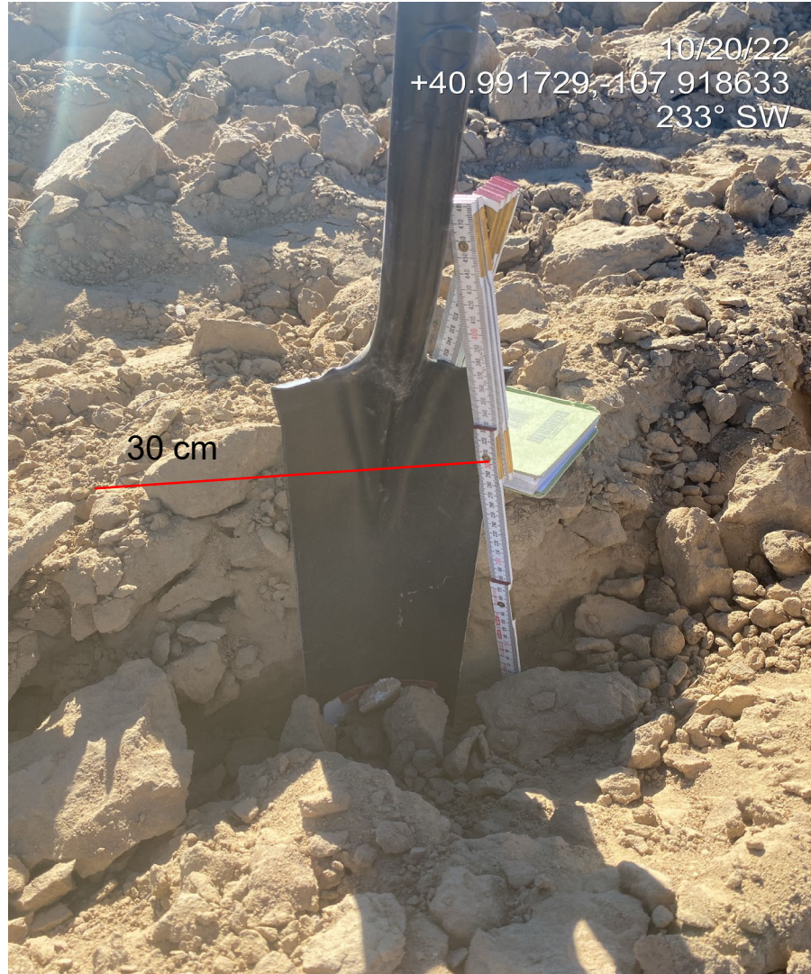
Photo 5. Photo shows the maximum depth of shovel penetration on the ripped interim area is 30 cm (12 inches). Some areas appeared to be ripped shallower.
