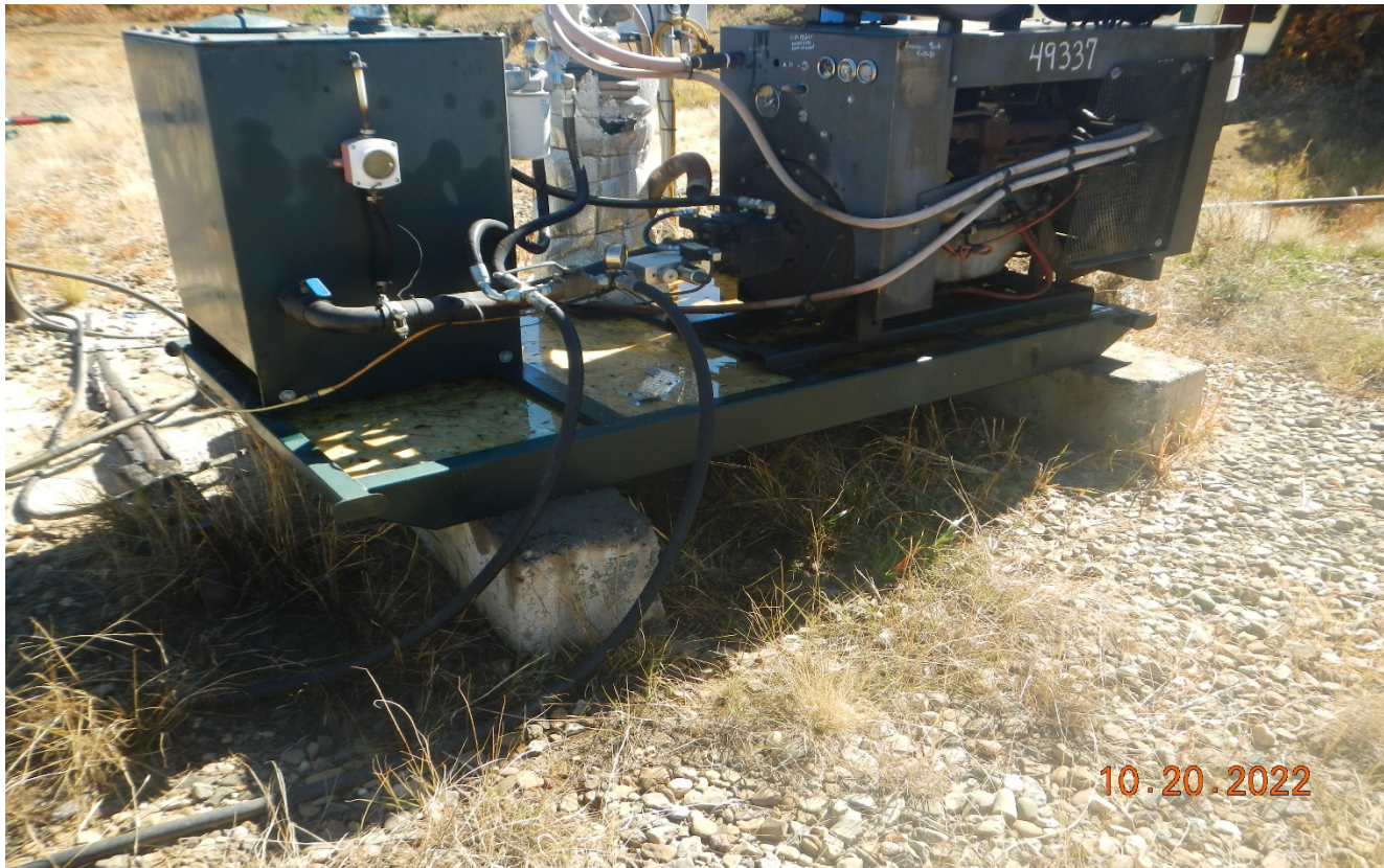
Photo 4. There is oily fluid in the engine skid that needs to be cleaned up.
