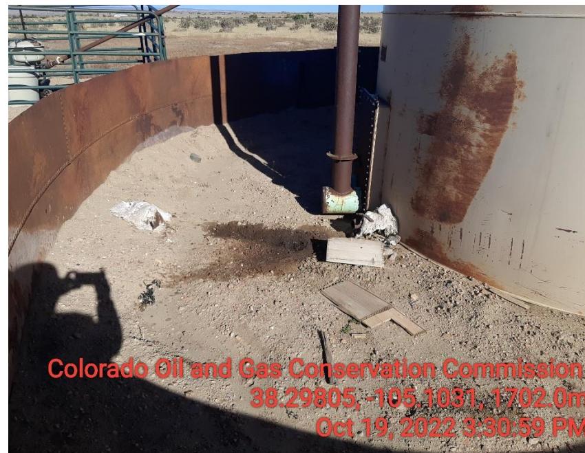
Photo 4 Stained soil Crude oil load out line. Mechanical issue
