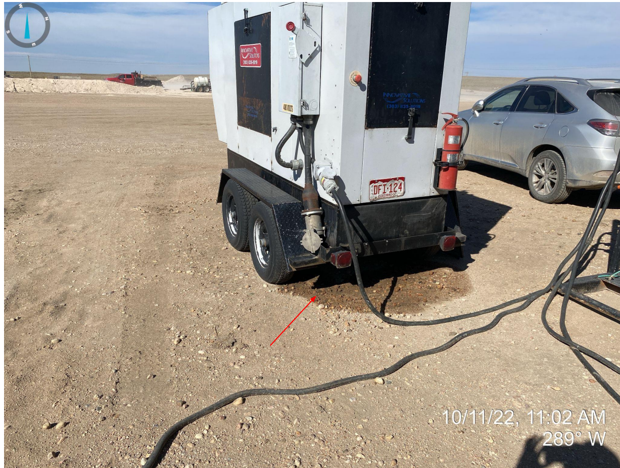
Photo 17. Taken near work trailers, facing west. Photo depicts stained soil underneath diesel generator, indicated by red arrow.
