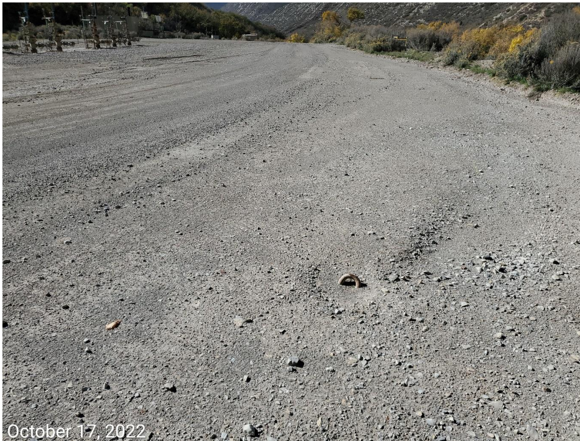
Photo 2: Photo shows example of unmarked anchor observed on Location.
