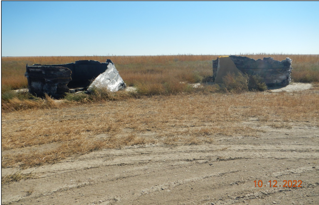
Photo 5. The burnt up tank remains at the east side of the location and needs to be removed ASAP.
