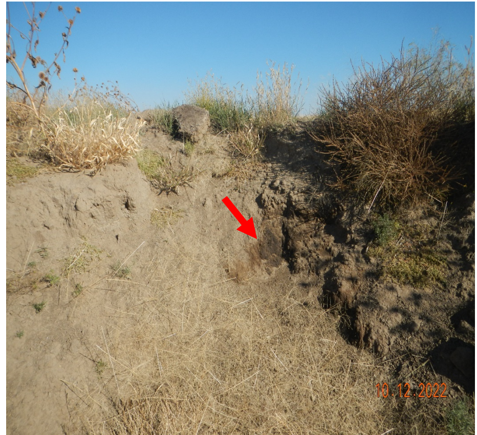
Photo 8. Located at the western side of the spill area. There is an excavated hole at this area approximately 12'x12'6'. There are still areas of oil stained soils at the surface (Bottom left) and 2ft. Down into the excavation area (right photo). Further excavation is needed.
