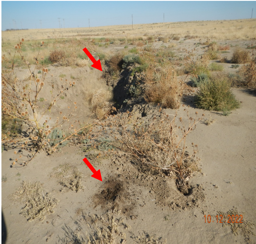
Photo 8. Located at the western side of the spill area. There is an excavated hole at this area approximately 12'x12'6'. There are still areas of oil stained soils at the surface (Bottom left) and 2ft. Down into the excavation area (right photo). Further excavation is needed.
