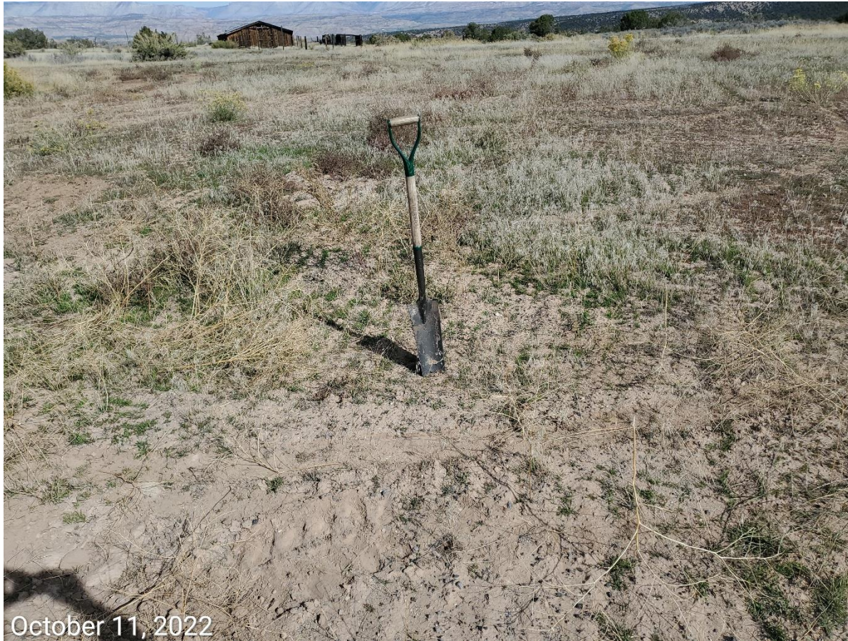
Photo 4: Reclamation Specialist attempted to conduct a soil compaction test pit on the Location. Photo shows compaction issues exist beginning at the soil surface; compaction alleviation has not been conducted on Location.
