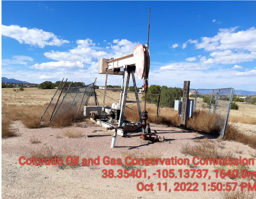
Photo 1 Well head. No well head sign
