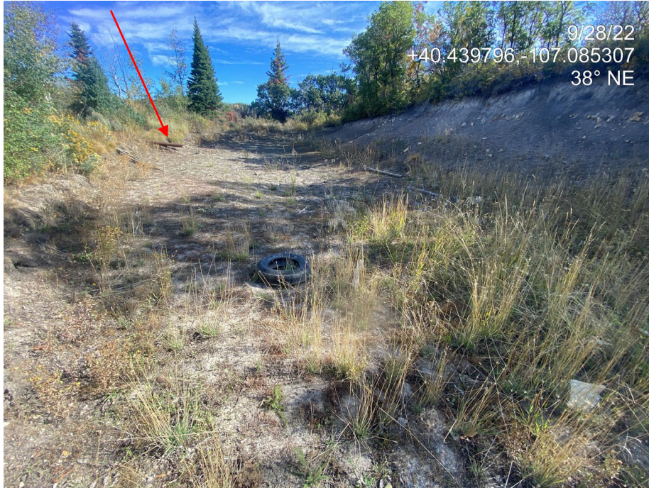
Photo 11. Photo taken from the northwest shows the center pit. Three former pits are unreclaimed. Note eroding cut slope, bare soil, trash and pipe (red arrow).
