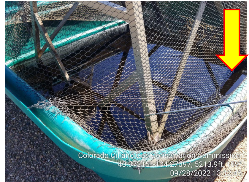
Photo 12 – Oil Waste in Containment and Netting in disrepair
