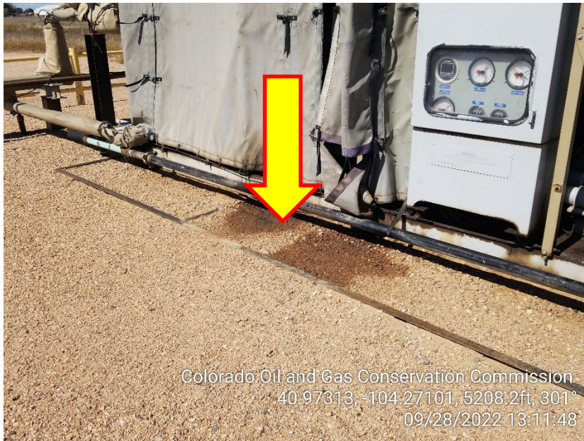
Photo 11 – Stained Soil at Compressor
