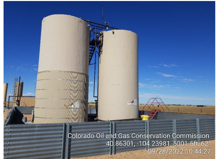
Photo 2 – Tank Battery
