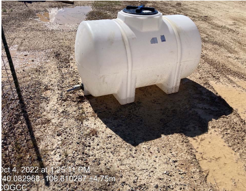
Tank not labeled or contained
