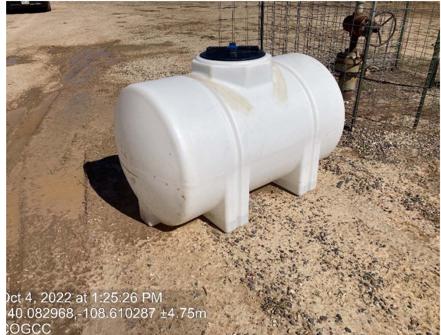
Tank not labeled or contained
