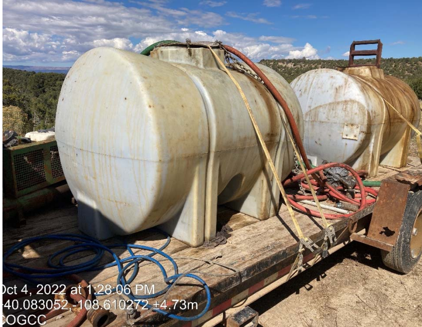
Tanks not labeled or contained
