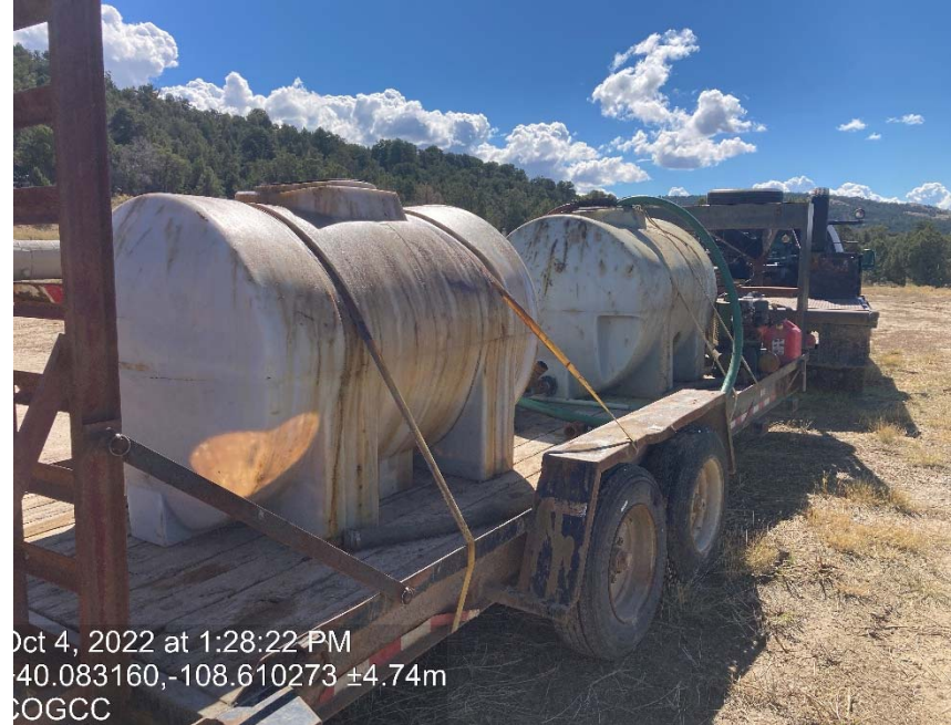
Tanks not labeled or contained
