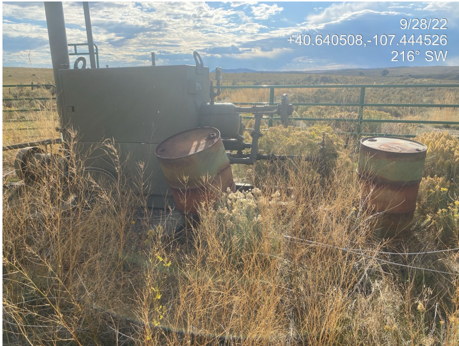
Photo 5. Photo shows containers without secondary containment.
