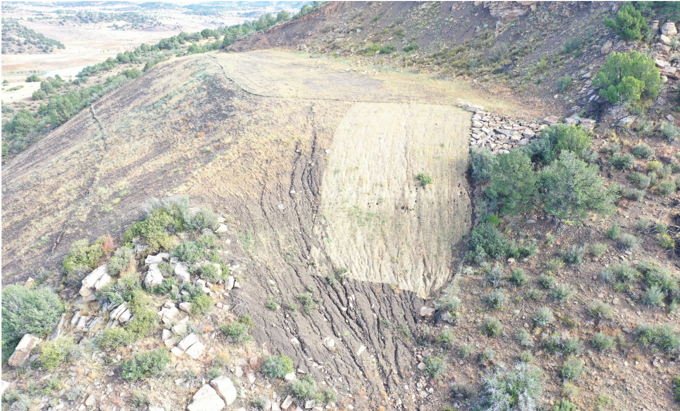
Photo 5. Facing north toward the location. There is rilling erosion that has not been repaired or controlled. There was erosion blanket installed on a portion of the slope however the rilling underneath the blanket is still evident and may continue to worsen.
