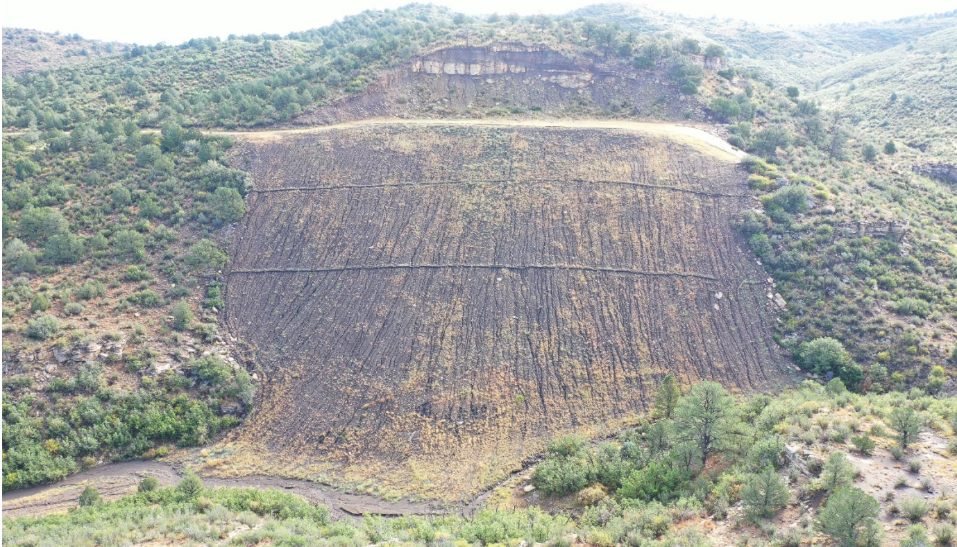
Photo 1. Drone aerial photo facing east toward the well site location. The access road and pad remain and were not recontoured back to the original condition per the rules. There has been significant erosion that has occurred.
