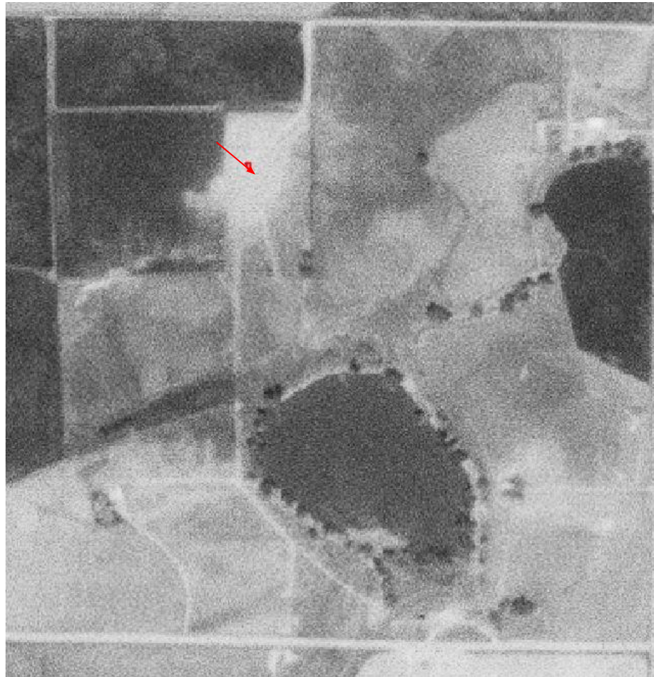
Photo 3. Historical imagery taken circa 1975. Image illustrates oil and gas operations under construction based on spud and completion dates (01/09/1975 and 05/26/1975, respectively) from scout card with larger surface disturbance. Red arrow indicates approximate well location.
